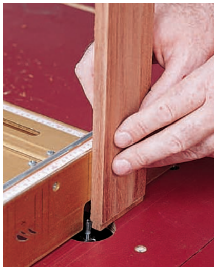
Figure 4: Use a 14° dovetail bit to form the joints on the drawer sides, fronts and backs.
