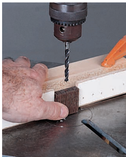
Figure 2: A simple jig facilitates drilling a series of accurate holes for the dowels that hold the chessboard grid together.
