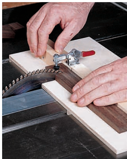
Figure 1: This crosscutting jig rides in the miter gauge slots of your table saw and is equipped with a toggle clamp to keep your fingers out of harm's way.
