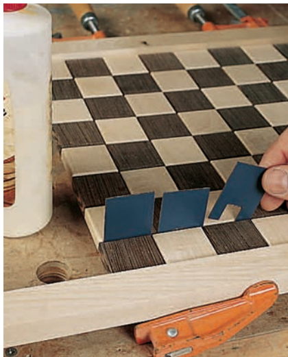
Figure 3: Use several plastic-laminate spacers to assure proper alignment when gluing up the squares of the chessboard. Cut a recess in each spacer to fit around the grid pin dowels.
