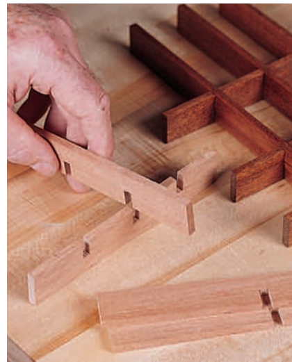
Figure 5: The drawer dividers are ripped and jointed to the correct width and thickness, then held together by half-lap joints.
