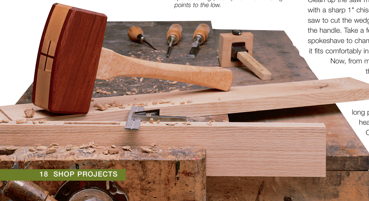
A comfortable handle is the key to a successful mallet. To reduce tearout while spokeshaving (above) work from the high points to the low.
