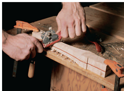
A comfortable handle is the key to a successful mallet. To reduce tearout while spokeshaving (above) work from the high points to the low.
