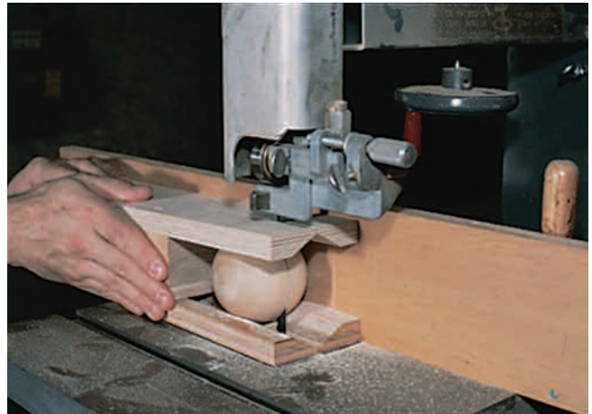
Figure 4: Use a V-jig for cutting the maple balls in half, making sure the ball fits very tightly. Cut slowly and stop the saw when the blade exits the ball, then reach in and remove the two halves.
