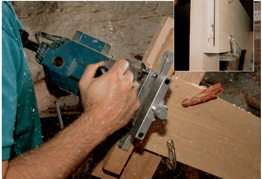
Figure 3: Hold the side rail in a bench vise while routing the bed rail fastener mortises. Clamping a scrap board flush with the rail's end stabilizes your router during this cut. Remember, you also need to cut two deeper channels within the mortise with a 1/4" bit so the fasteners lay flat.
