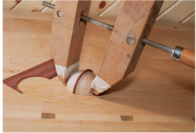
Figure 6: A wooden handscrew clamp works well to assemble the ball caps. Tape a folded piece of sandpaper to the ends of both jaws to get a better grip and to protect the maple ball sections.
