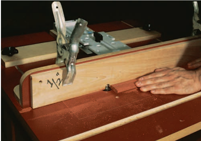
Figure 1: Round over the edges on the padauk slats by raising the 1/4" bit so the outside tip of its curve is even with the table surface. Align the face of the fence with the outside edge of the bit's bearing.
