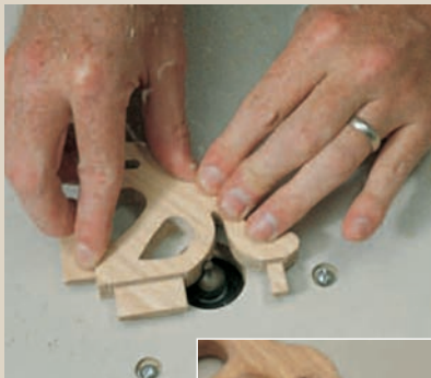
Round over the scroll sawn edges of the brackets with a piloted 1/4"-radius roundover bit in a table-mounted router.
