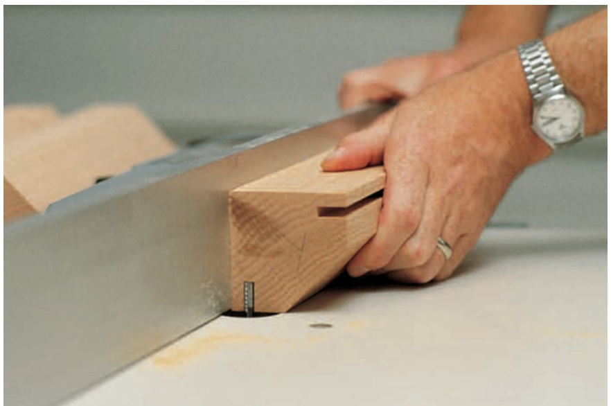
Figure 1: Mortises in the legs (they house tenons on the brackets and aprons) are cut on a router table using a 1/4" spiral-fluted straight bit.
