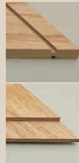
Use your table saw to create tongues on the short sides of the triangular bracket blanks, as shown in the two photos at left. Begin by making a pass to define the tenon (using a sharp blade to combat tearout), then remove the rest of the waste in subsequent passes.
