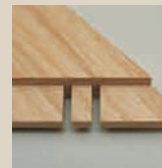
After changing the blade height, use your miter gauge to complete the tenons. The waste between them will be replaced by fillers (pieces 8) during assembly.
