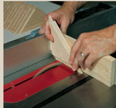
After changing the blade height, use your miter gauge to complete the tenons. The waste between them will be replaced by fillers (pieces 8) during assembly.
