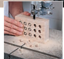
Figure 6: You can cut your own screw hole plugs with a 3/8" plug cutter in your drill press. Cut the plugs loose by resawing to 3/8" on your band saw.
