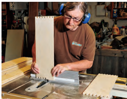
A box joint jig is used with the table saw to cut all the joinery for the drawer boxes. The jig's reference pin spaces the cuts for a snug fit.
