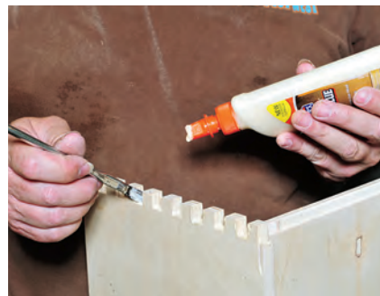
To assure a strong drawer, brush a thin layer of glue onto all mating surfaces of each corner joint. A disposable flux brush is used here.
