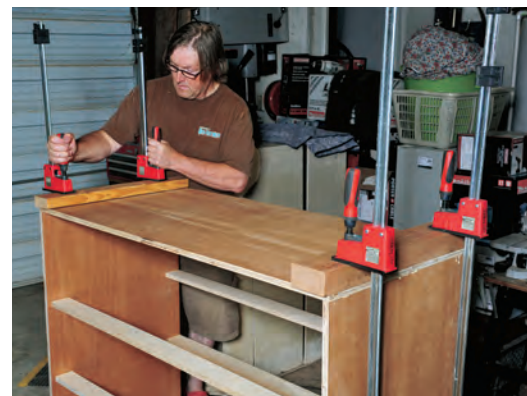
The second step in assembling the carcass is to glue and clamp the top onto the sides, using cauls to distribute the clamping pressure.
