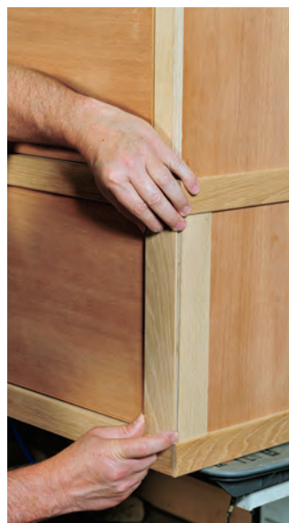
Thin red oak slats (at far left) are glued and nailed to the carcass sides, top and front, to enhance the dresser's trunk-like appearance. Thinner wood strips glued and nailed on vertically define the trunk dresser's edges and protect and hide the bare plywood edges (near left).
