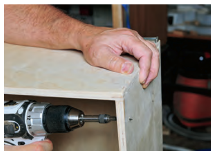
At left, plywood spacers glued to the inside of the carcass provide a mounting surface for the dresser's full-extension drawer slides. To mount the drawer faces, screws are first partially driven through the drawer box fronts (above). With the drawers mounted on their glides, each drawer face is set in place, then tapped from behind (right top). The screws are then fully driven to secure the face (right bottom).
