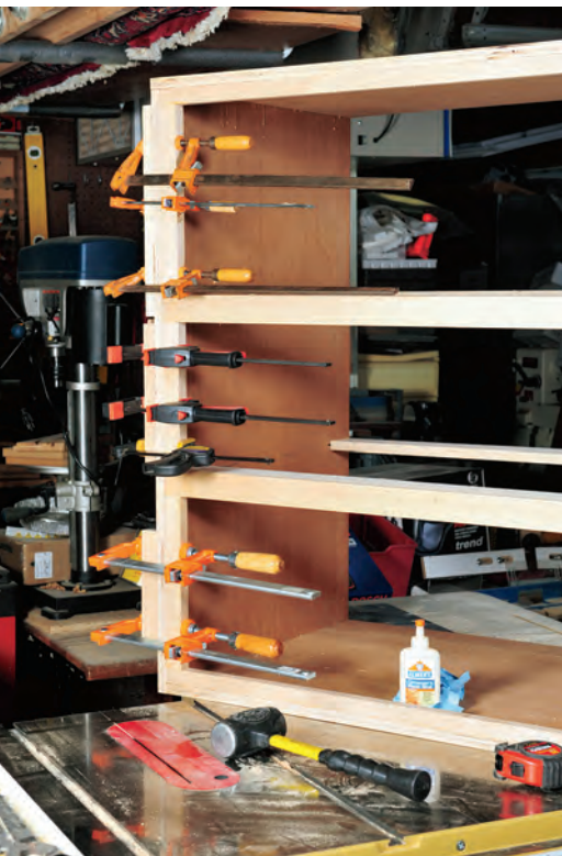
Face frame members are glued in place into the carcass flush with its front edges. Joinery may be added, but it isn't absolutely necessary.
