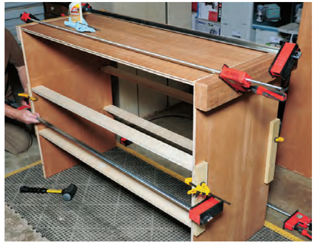
Above left, the author uses a biscuit joiner to plunge-cut slots that join the parts of the dresser carcass. A marked stick (at left) is used to help space the biscuit slots evenly. The carcass sides, bottom and stretchers are glued and assembled at one time (above right).
