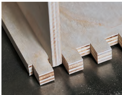
The slot for the drawer's bottom is located in between two of the pins, so that the slot will be hidden on the drawer's sides.
