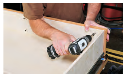
At left, plywood spacers glued to the inside of the carcass provide a mounting surface for the dresser's full-extension drawer slides. To mount the drawer faces, screws are first partially driven through the drawer box fronts (above). With the drawers mounted on their glides, each drawer face is set in place, then tapped from behind (right top). The screws are then fully driven to secure the face (right bottom).
