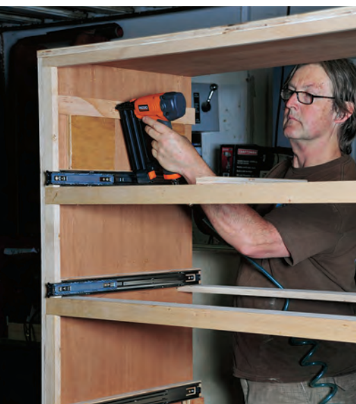
At left, plywood spacers glued to the inside of the carcass provide a mounting surface for the dresser's full-extension drawer slides. To mount the drawer faces, screws are first partially driven through the drawer box fronts (above). With the drawers mounted on their glides, each drawer face is set in place, then tapped from behind (right top). The screws are then fully driven to secure the face (right bottom).
