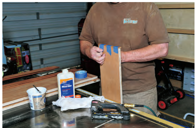
Thin solid-wood edging is glued and taped onto the edges of the separately mounted drawer faces, to cover up the bare plywood.
