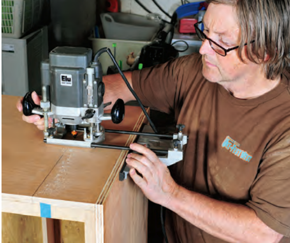
The author uses a router fitted with a V-bit and an edge guide to rout a shallow groove on the side of the carcass, to make the steamer trunk dresser appear to have a liftable lid.
