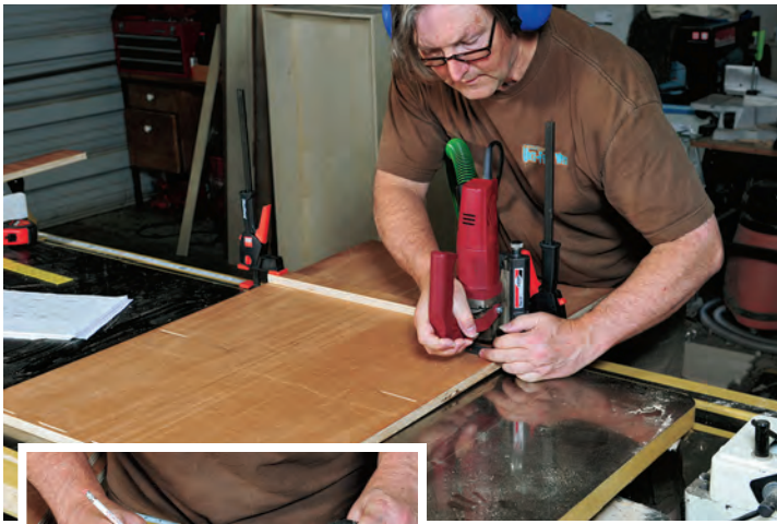
Above left, the author uses a biscuit joiner to plunge-cut slots that join the parts of the dresser carcass. A marked stick (at left) is used to help space the biscuit slots evenly. The carcass sides, bottom and stretchers are glued and assembled at one time (above right).
