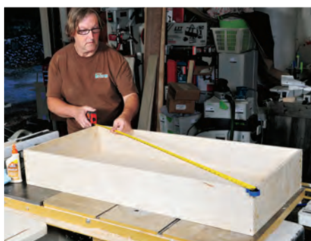
After gluing and assembling the drawer's back and two sides, slide the drawer bottom into its slot before fitting the front piece in place. Before clamping up the drawer box, set it on a flat surface and check it for square by making sure it measures the same from corner to corner (inset photo).
