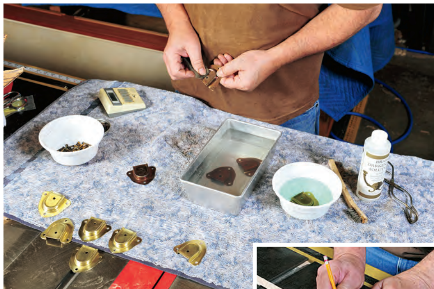
Dipping shiny hardware in a special brass darkening solution (above) gives them an antique brass appearance. The wood lid lipping strip on the front of the dresser (right) must be trimmed to fit around some hardware components.
