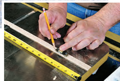
Dipping shiny hardware in a special brass darkening solution (above) gives them an antique brass appearance. The wood lid lipping strip on the front of the dresser (right) must be trimmed to fit around some hardware components.
