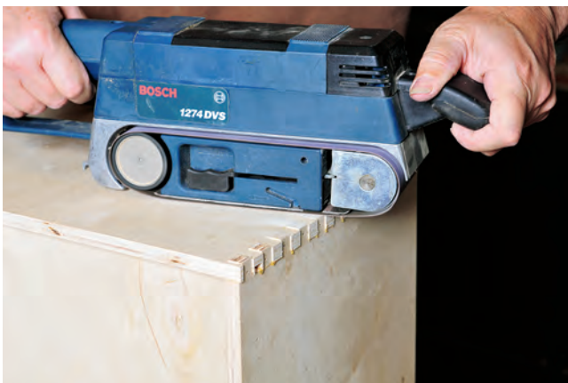
A belt sander makes quick work of trimming the overhanging pins flush at all the corners of each Baltic birch plywood drawer box.
