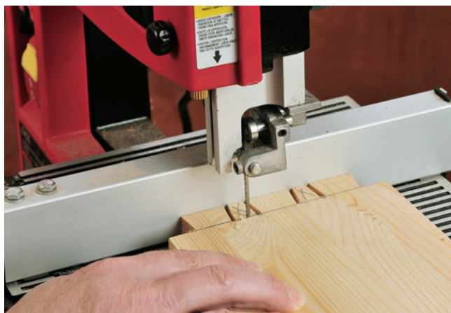
Figure 11: An efficient way to remove the waste between tails is to use your band saw equipped with a narrow saw blade. Set the fence to the proper distance and carefully saw away the waste.
