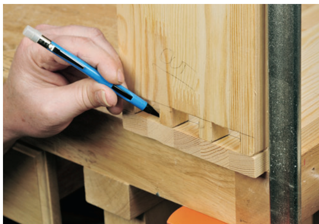
Figure 9: Mark out the tails on the tail board using the pin board as shown in the photo. Use a square to mark the depth of the tails. The process is similar to marking out for hand-cut dovetails.
