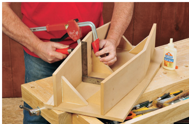
Figure 3: Braces keep the tail fence perpendicular to the base.
