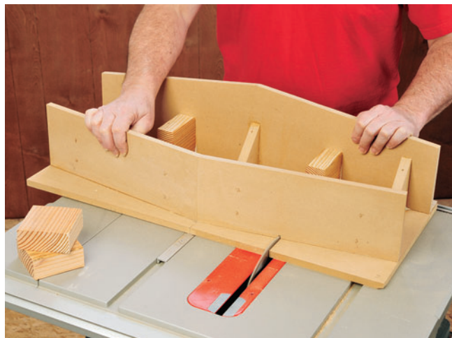
Figure 5. "Cutting in" a registration slot on all four of the jig's fences is essential for locating your dovetail cuts. Note the freshly glued-in blocks of wood: these cover the saw blade's exit points and protect your fingers.
