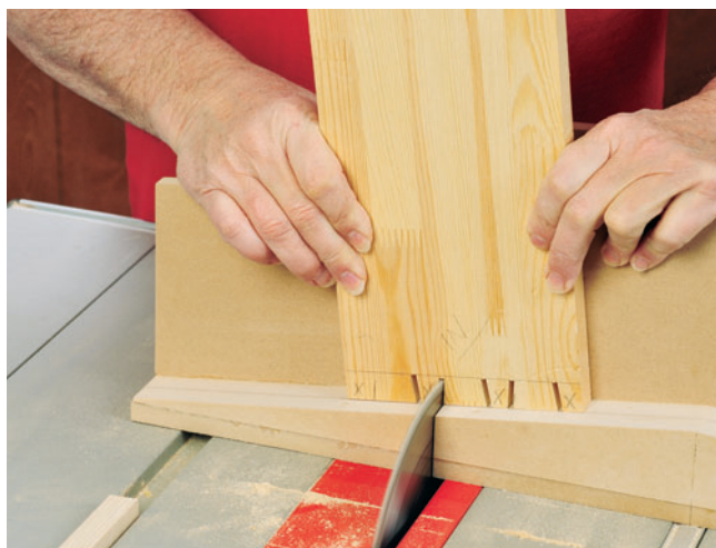
Figure 10: Spin the jig around front to back and cut the tails, using the ramps on each side of the jig to make the right- and left-hand cuts.
