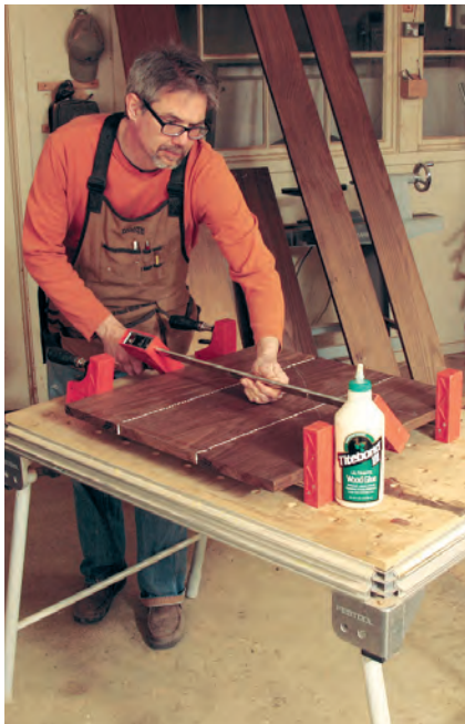
The chair's back and the seat (above) were both laminated using a waterproof glue. The thermo-treated oak requires longer clamp time.
