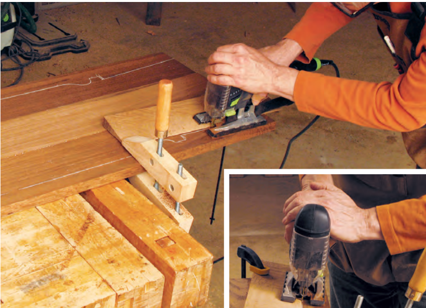
The symmetrical taper at the bottom of the back also has a 12° angle across its thickness. A ramp cut to the proper angle was clamped in place and used to form both angles in a single cut.
