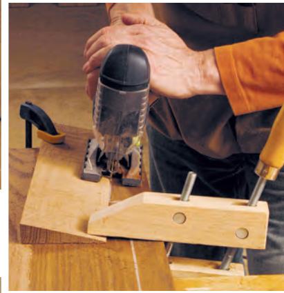
The symmetrical taper at the bottom of the back also has a 12° angle across its thickness. A ramp cut to the proper angle was clamped in place and used to form both angles in a single cut.
