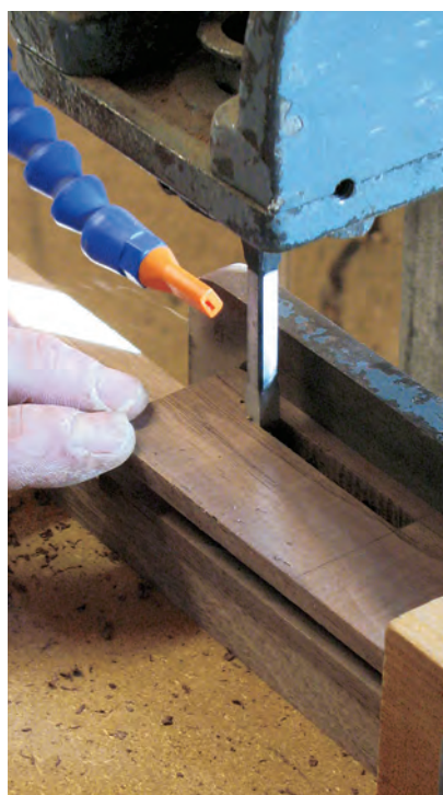
Chopping the mortises with his dedicated mortising machine, the author prefers to start with the innermost cut, working his way out. This helps to avoid bit deflection.
