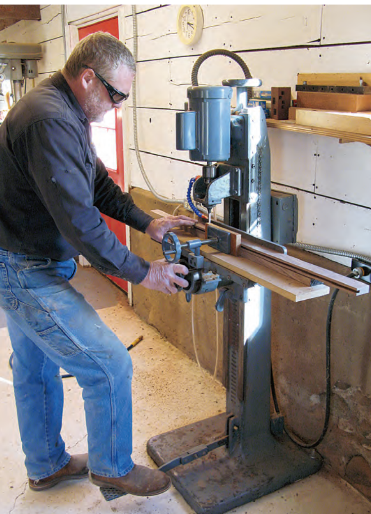
Chopping the mortises with his dedicated mortising machine, the author prefers to start with the innermost cut, working his way out. This helps to avoid bit deflection.
