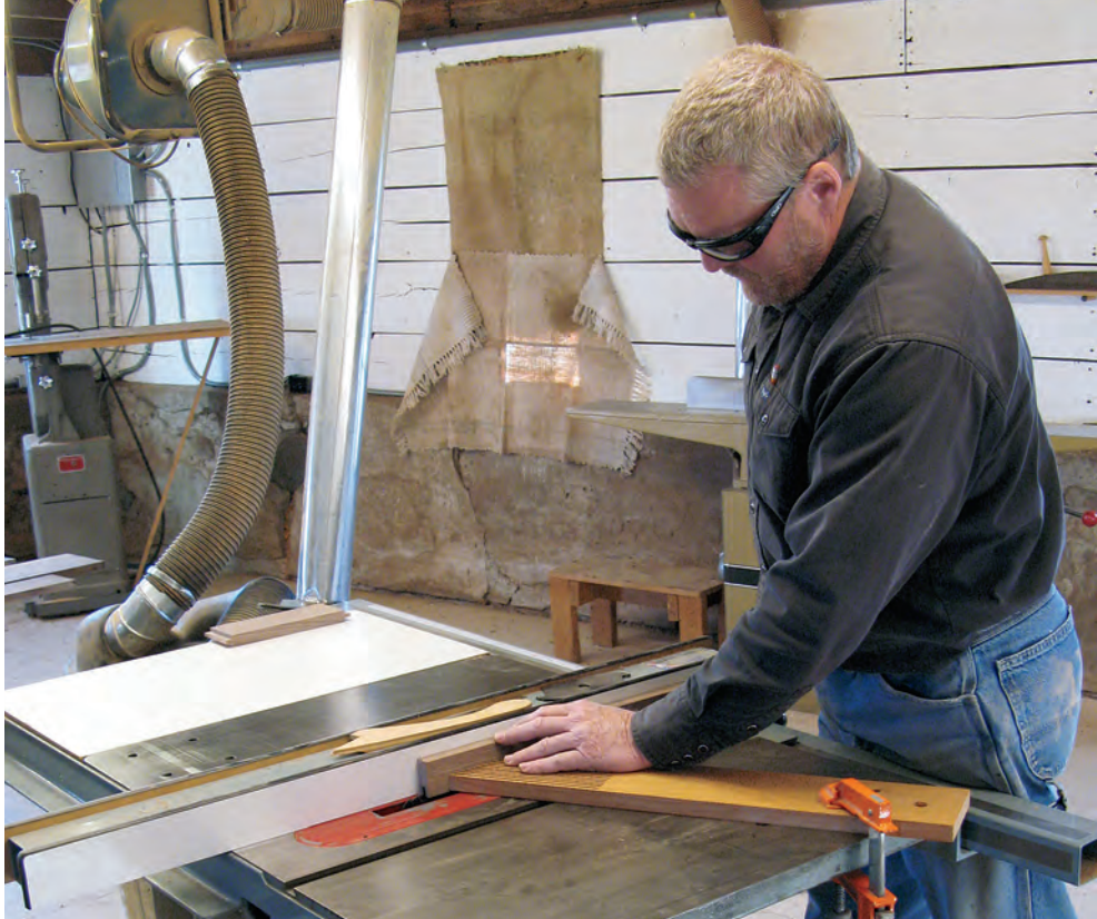
The author used a table saw with a narrow dado head to plow the grooves in the stiles and rails. His shop-made featherboard helped keep the stock tight to the fence as he made the cut.
