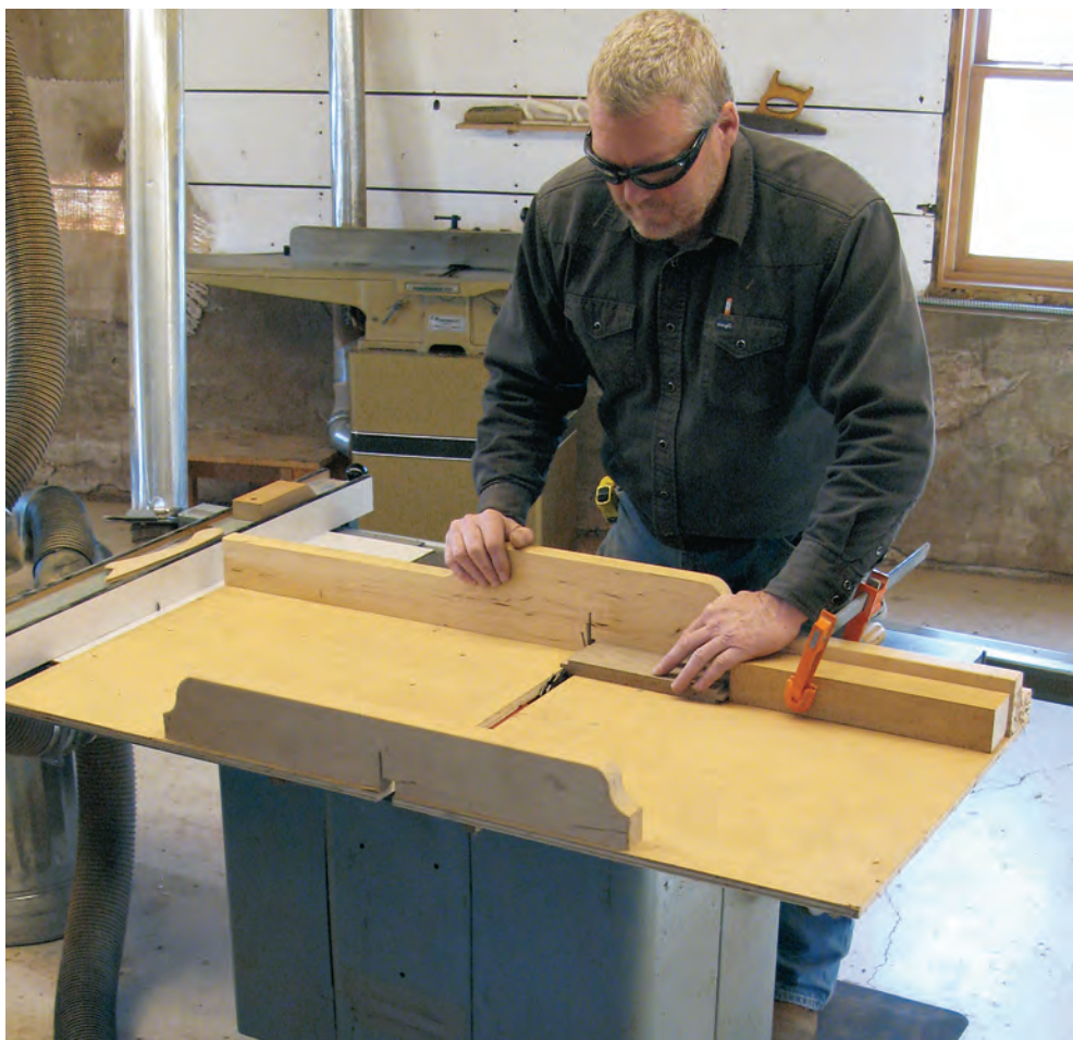
The author used his large crosscut sled to form the tenons on the rails, gaining additional accuracy and repeatability by clamping a stop block to the jig. As can be seen from the position of his hands, this approach also significantly increases the operation's safety.
