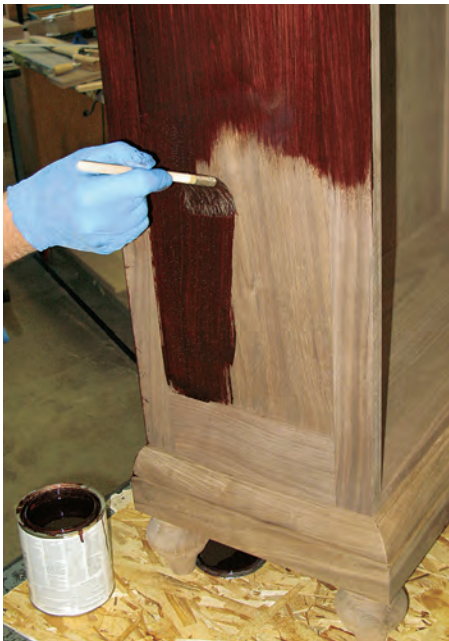
Red mahogany oil stain (left) added colorful highlights to the walnut lumber — popping the grain nicely. Above, the ends of the shelf (turned around so you can see the back) have a groove sliced into them that slides over the winged shelf pins.
