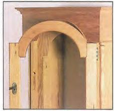
The hood molding is applied around the completed hood, but is notched at the back so the hood wings (KK) can run by. The wings are 1/4 in. thick stock and notched to fit around the hood back rail and over the waist molding (F). The wings are screwed to the gallery sides and the hood side collars.
