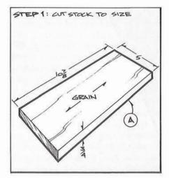
Step 1: Cut four pieces of <sup>3</sup>/<sub>4</sub> in. thick stock to 5 in. wide by 10<sup>7</sup>/<sub>8</sub> in. long.
