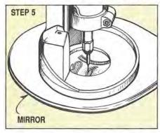
the <sup>1</sup>/<sub>16</sub> in. solid carbide inlay bit. The bit depth of cut is set just a hair under the pearl thickness, allowing the pearl to stand a little proud of the ground's surface. Note that on our bit we had to grind the end of the shank back slightly to get the proper depth setting in the collet.
