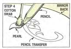
best to have the ground—in this case the back of the mirror—clamped securely to your bench top so it won't be moving about as you trace the pearl.
