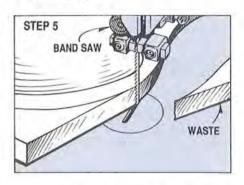
Step 5: Cut the outside profile. Use the band saw, handheld jigsaw or a coping saw. Use files to smooth any irregularities and remove the saw marks. It's important that the edge be smooth for the next step.
