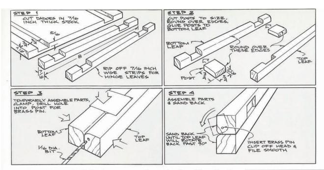
back of the hinge, gradually the degree of pivot will increase, until the hinge opens just past 90 degrees, as shown.
