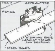
the work down solidly on the table directly over the cutter. In addition to preventing chatter at this critical area, it also provides some guarding of the cutter. I then clamp two or three feather-boards flat on the table, so they hold the work securely against the fence.
