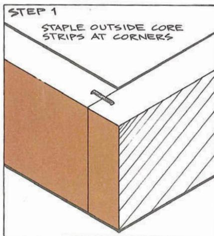
be a screw, dowel, bolt, etc., you must have solid core strips to support the attachment. You don't want a screw to be holding only to a  $\frac{1}{2}$  in. skin. So, at every location where something will be mounted, add extra core strips to the basic layout. Remember, keep it as simple as you can.
