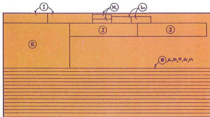
CUTTING DIAGRAM - FROM (2) 4 x 8' SHEETS MDF (1/2 INCH THICK)
