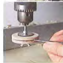
Figure 2: Make a wheel sanding jig from a 3/16" threaded rod, a nut, two rubber-backed washers and a wing nut. Use the jig to score the wheels for their O-rings, too.
