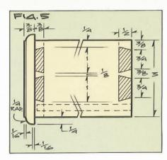
any glue that may have squeezed out and sand the joint smooth. Now, drill and counterbore on each end for two 1<sup>1</sup>/<sub>2</sub> in. long by no. 8 flathead woodscrews.
