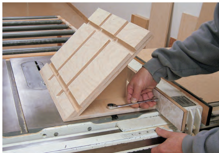
Use your saw's fence to align the jig parallel to the saw's blade. Mark the location of the miter bar on the jig ends. Locate and drill its holes and then attach the miter bar with a wrench, as shown here.
