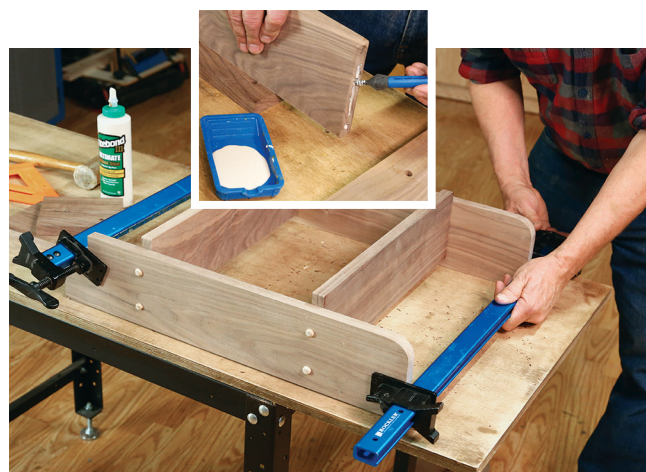
To assemble the self carcass, start by attaching one side to both shelves. Apply glue in the shelf holes, slide the pegs through the side and push the pieces together. Do the same for the other side and then clamp it together.
