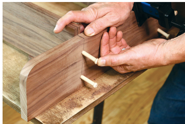
As you bore the holes, temporarily insert the pegs. They are too long to fit properly, but they will hold the parts in alignment. This is essentially a dry or test fit. Boring holes for each shelf must be done separately.
