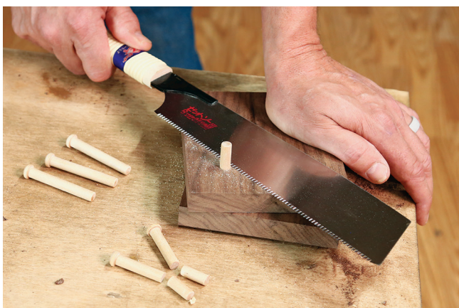
Easily cut the pegs to length by drilling a 3/8" hole through the two 3/4" walnut waste pieces, then slide a peg through and saw it to length as shown. This leaves the barrel of the peg 1 1/2" long.
