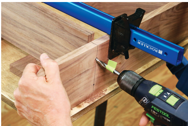
With the top shelf clamped in place, bore 3/8" holes through the sides into the ends of the shelves. The shelf is held up by a 3/4"-thick scrap. The drill bit is wrapped with masking tape at 2" from the end to set the hole depth.
