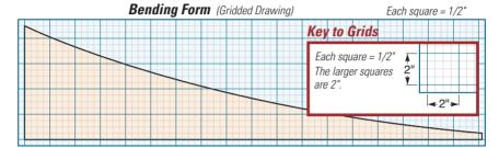
The drawing above shows the shape of one of the 361/4"-long, 9"-high segments that make up the bending form. You'll need to cut out seven of these to properly build the form.
