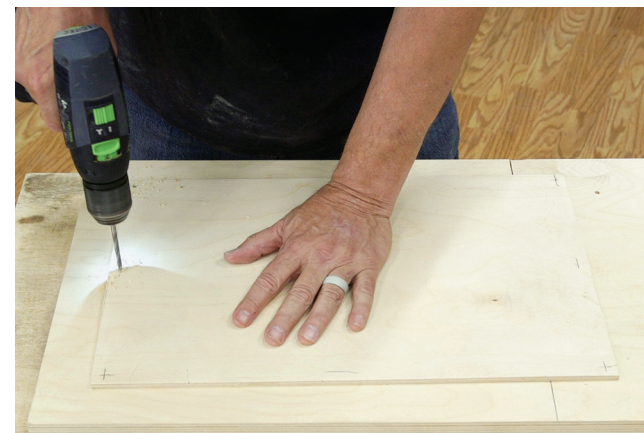
Attach the door panel to the back of the door frame with eight screws. Sand the plywood smooth. Mount the panel, then remove it to apply your finish of choice.
