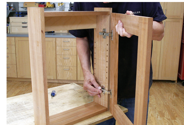
The door snaps easily into place on the hinge clips. Adjusting screws on the hinges will then allow you to fine-tune the position of the door frame relative to the carcass. That's a primary benefit of Euro-style cup hinges.
