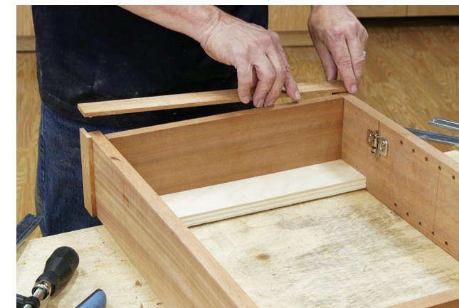
The decorative trim is simply cut to length and glued to the outside top of the carcass. When the glue cures, sand the carcass smooth and apply your finish of choice.
