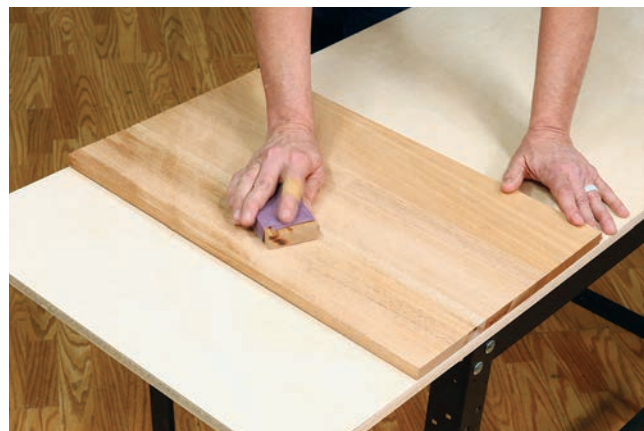
Photo 8: Starting with 80-grit paper, sand diagonally across the panel. Then sand diagonally the opposite way with 100-grit to remove all the 80-grit scratches. Finally, switch to 150- and 180-grits, and sand lengthwise.
