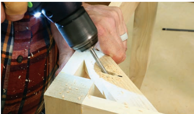
Photo 13: Drill three \frac{3}{16} "-diameter holes in a line in each angle brace, parallel to the short aprons. Then angle the drill to connect these holes.
