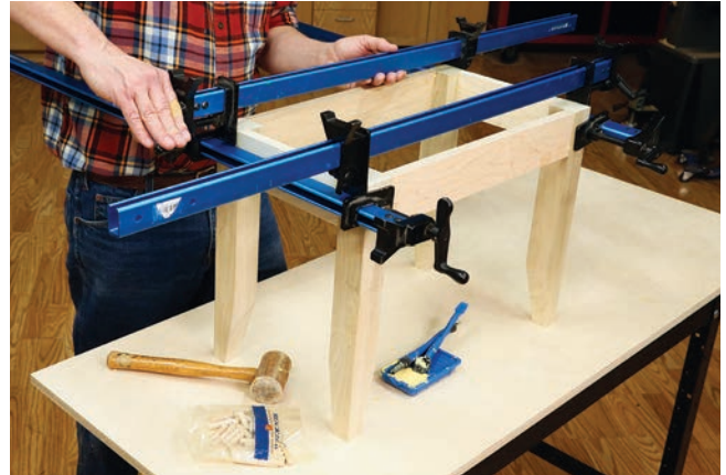
Photo 10: Apply glue to the dowels and the ends of the aprons. Tap the pieces together with a mallet, if necessary. Clamp the leg and apron subassembly together and allow the glue to cure.
