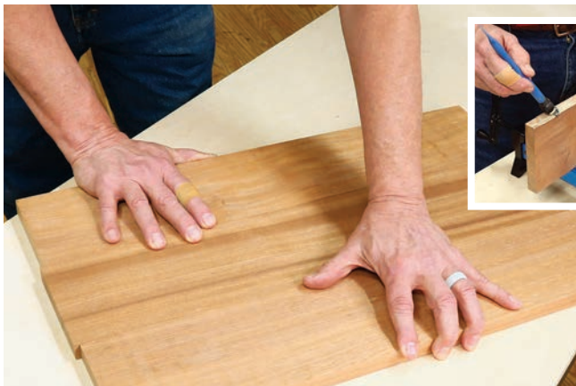
Photo 5: Arrange the three tabletop pieces in a way that uses the figure of the wood most attractively. (This is entirely subjective.) Mark them in some way to keep the orientation of the boards clear.
