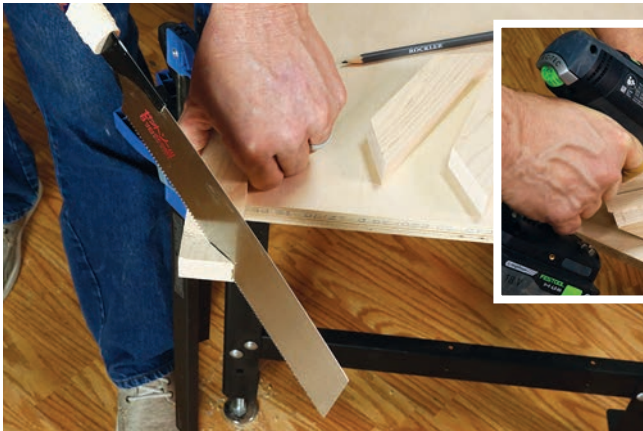
Photo 11: From the remaining apron stock, rip and crosscut 1\frac{1}{2} " x 6\frac{1}{2} " pieces to make the angle braces. Use a speed or combination square to mark 45-degree angles on each end, and cut these mitered corners.
