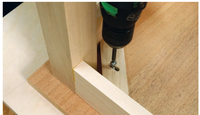
Photo 14: Attach the tabletop to the leg and apron subassembly using the same screws as in Photo 12. Snug up the screws but do not overtighten.
