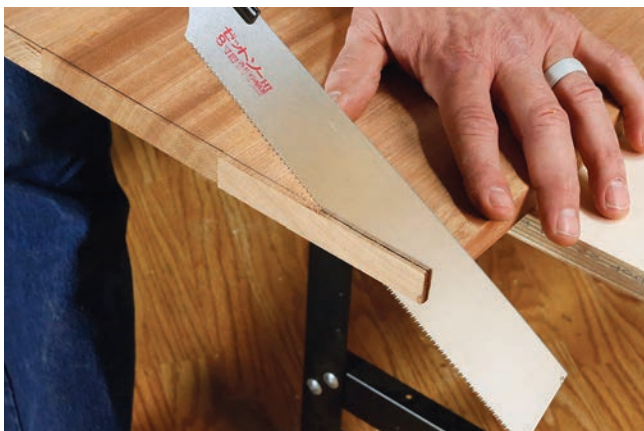
Photo 7: Use a square of some type to draw a line across the tabletop near each end. Trim off these waste areas with a handsaw. Smooth the cut ends with sandpaper and a sanding block, removing any saw marks.
