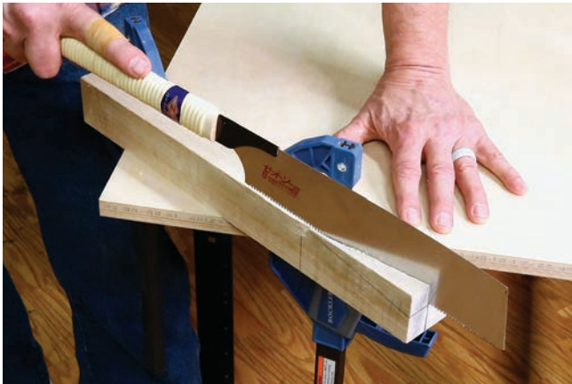
Photo 1: Measure in 1\frac{1}{8} " at the bottom of the leg and 4\frac{3}{4} " up the edge of the leg to form a long narrow triangle. Use your hand saw and the techniques from our last Woodworking Basics article to cut the section away.
