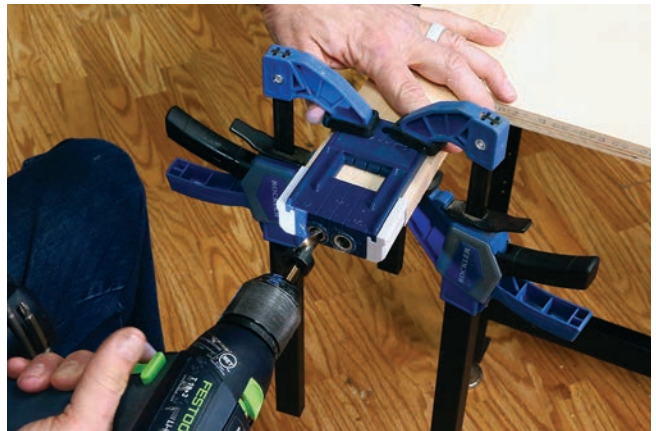
Photo 4: Center the doweling jig on the ends of the aprons and bore matching holes to the ones you just drilled into the legs.
