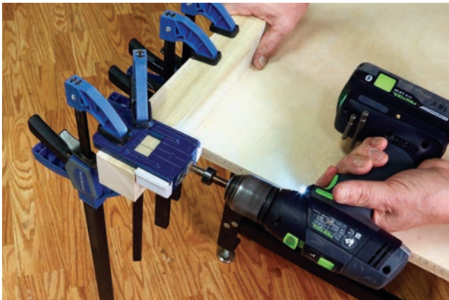
Photo 3: Mark a line 1\frac{1}{2} " down from the top of a leg. Use that line to locate a doweling jig set up for 3/8 " dowels. Use the Drawing below to position the dowels on the proper faces. Drill two dowel holes per leg face.
