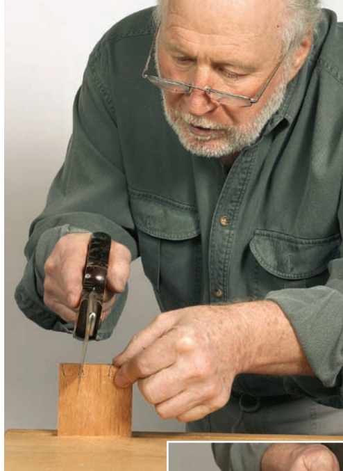
Cutting the tails for a single-lap dovetail is the same as cutting the tails for a through dovetail. After cutting the tail slopes with a dovetail saw, remove the bulk of the waste with a coping saw. Your next step is to clean up to the lines by vertical and horizontal paring.
