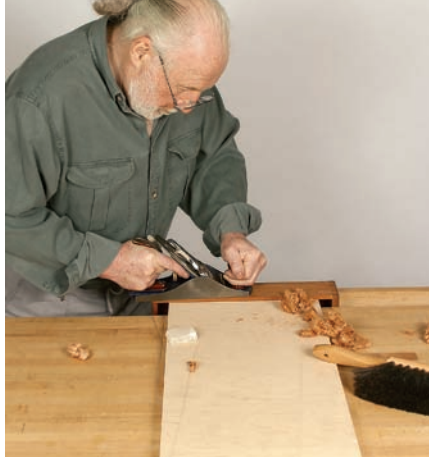
Plane both drawer sides down to match the end grain of the dovetail pins.
