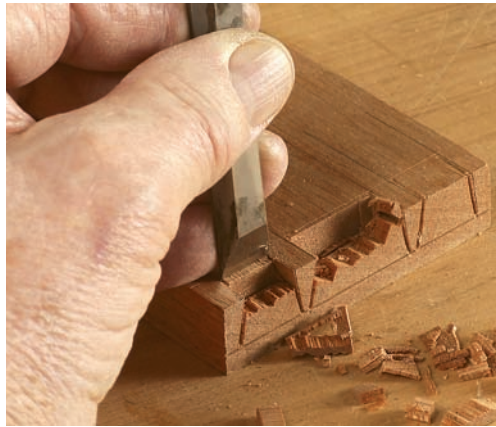
After cutting with a dovetail saw, lay the front on your bench and begin chopping out the waste across the grain
