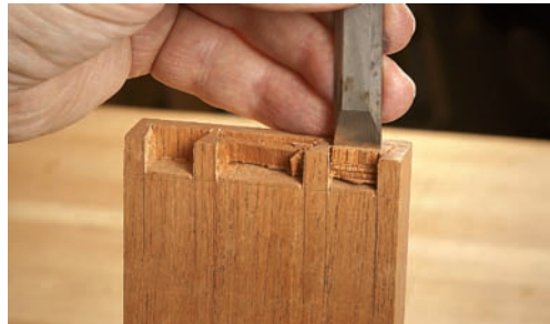
Next, clamp the drawer front in the vise and continue chopping out the waste down the grain.
