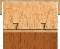
Use the tails to mark the pins by positioning their ends up to the lap gauge line. After you've completed step 5 (above) trial fit the joint. Note the drawer side stands proud of the ends of the pins (inset).
