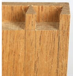
The corner waste is removed by first severing the end grain with a pair of purpose-made 1/4" skew chisels. The goal is pins and sockets that are clean as a whistle.
