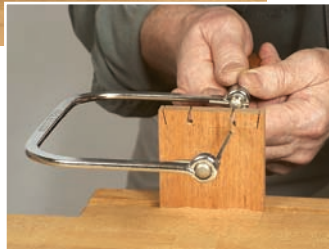
Cutting the tails for a single-lap dovetail is the same as cutting the tails for a through dovetail. After cutting the tail slopes with a dovetail saw, remove the bulk of the waste with a coping saw. Your next step is to clean up to the lines by vertical and horizontal paring.
