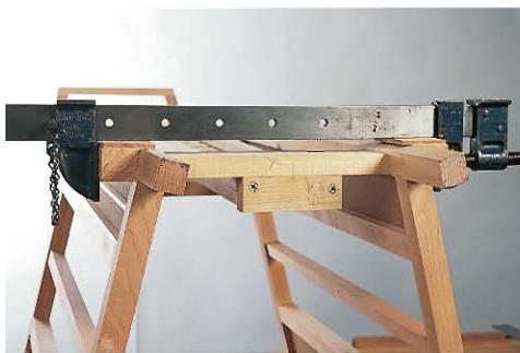
Angled clamping blocks compensate for the shoulder line angle. The addition of a plywood pad helps hold the block in position and protects the workpiece.
