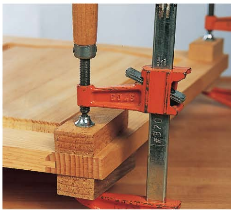
The only way to apply pressure to the gluing surfaces of a mortise-and-tenon joint is by clamping across the joint faces.
