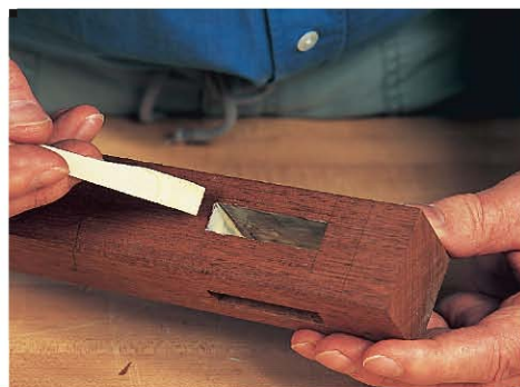
A paddle can be custom-shaped to apply glue effectively to hard-to-reach surfaces.
