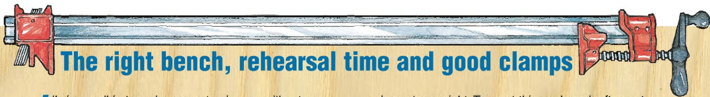
The only way to apply pressure to the gluing surfaces of a mortise-and-tenon joint is by clamping across the joint faces.
