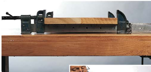
Too much pressure can bow a flat panel. Use a straightedge to check for flatness (inset). If it is bowed, reduce pressure and alternate clamps top and bottom.
