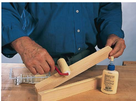
A trim roller is ideal for edge joints. Load the roller in the tray, then spread to uniform thickness.
