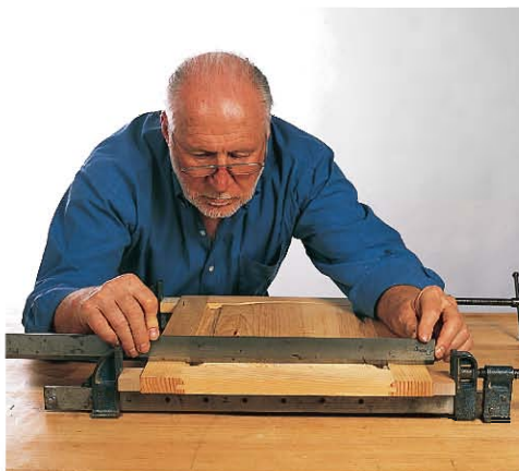
The clamping blocks and checking procedure for gluing up a door are the same as for a mortise-and-tenon.
