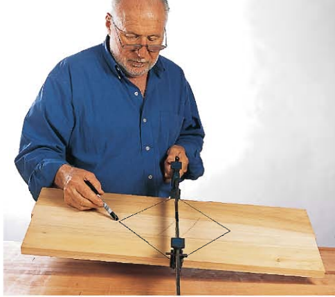
Clamping pressure fans out from the clamp heads at 45° in each direction and is transmitted to the glue line as indicated by the author.
