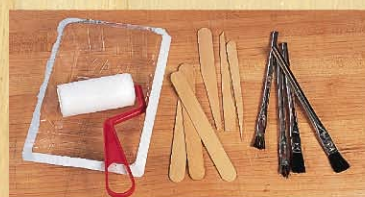
Three types of glue applicators that will cover most gluing requirements: roller, paddle, and brush.
