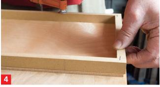
4. Align and clamp the core frame on the first skin using your fingers as the measuring tools. The skin brings the frame into square. Note that the author has cut his skins so that a bare 1/32" overhang occurs.
