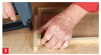
3. Join the core frame with staples top and bottom as previously described. MDF has a tendency to blow out or fracture when stapled. Take extra care to place the staples in the center of the material.
