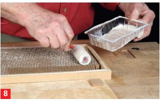
8. Roll glue on the Tricel core. The high rag content in the Tricel provides thousands of fibers that will bond to the skin, but the fibrous material also soaks up glue. Roll out a sufficient amount to transfer.
