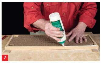
7. Lay a strong line of glue on the frame. A bit of squeeze-out is not only acceptable, but necessary, to provide confidence that the seam has sufficient glue coverage to bond properly.
